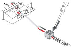
4. Use #1 Phillips to loosen the 4 terminal screws on 8MM-EZ Connector. Peel 1/2" of the adhesive protector from back of LED tape light, and scrape waterproof coating, insert into connector, evenly tighten screws. Insert wires from WAV Smart Receiver / Power Supply into terminals, Red wire to (+ or WW) side of tape, Black wire to (- or CW) side of tape; tighten screws.
