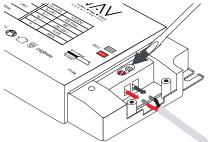
3. Insert one end of stripped wires into WAV Smart Receiver LED Terminals, Red wire to (WW+) and Black wire to (CW-) terminals. Tighten screws.
