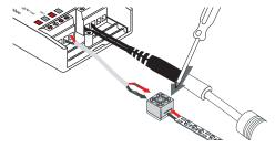
4. Use #1 Phillips to loosen the 4 terminal screws on 8MM-EZ Connector. Peel 1/2" of the adhesive protector from back of LED tape light, and scrape waterproof coating, insert into connector, evenly tighten screws. Insert wires from WAV Smart Receiver into terminals, Red wire to (+ or WW) side of tape, Black wire to (- or CW) side of tape; tighten screws.
