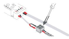
3. Use #1 Phillips to loosen the 4 terminal screws on 8MM-EZ Connector. Peel 1/2" of the adhesive protector from back of LED tape light, and scrape waterproof coating, insert into connector, evenly tighten screws. Insert wires from Wired Controller into terminals, Red wire to (+ or WW) side of tape, Black wire to (- or CW) side of tape; tighten screws.
