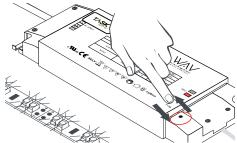
2. If setting WAV Smart Receiver / Power Supply up for the first time, clear the memory by pressing and holding the "Prog" button until the lights blink twice.
