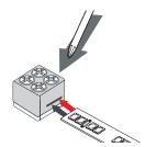
2. Use #1 Phillips to loosen the 4 terminal screws on 8MM-EZ Connector. Peel 1/2" of the adhesive protector from back of LED tape light, and scrape waterproof coating, insert into connector, evenly tighten screws.
