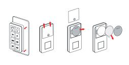
1. Remove Controller from back plate, slide battery compartment open, remove battery, and discard clear plastic tab. Reinsert battery, replace cover.
