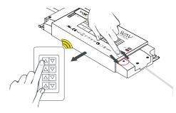
3. Very quickly, click and release the "Prog" button and, within 5 seconds, quickly click and release the "On Light Bulb" button on the Controller. When lights blink once, Controller and Receiver are paired.
