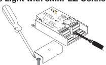
2. Use #2 Phillips to loosen screw and remove cover from WAV Smart Receiver. Use the flat head from the multi-bit screwdriver to loosen one terminal marked (CW-) and one marked (WW+).
