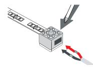
3. Insert stripped wires from WAV Smart Receiver into terminals, Red wire to (+ or WW) side of tape, Black wire to (- or CW) side of tape; tighten screws.
