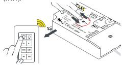
**5.** Turn on 120V AC to Power Supply and pair WAV Smart Receiver to Controller.
