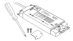
2. Use #2 Phillips to loosen screw and remove cover from WAV Smart Receiver / Power Supply. Use the flat head from the multi-bit screwdriver to loosen one terminal marked (CW-) and one marked (WW+).
